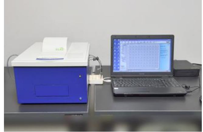
Microplate luminometer BERTHOLD CentoroXS3 LB960 Instrument for luminescence assays in 96-well plates
