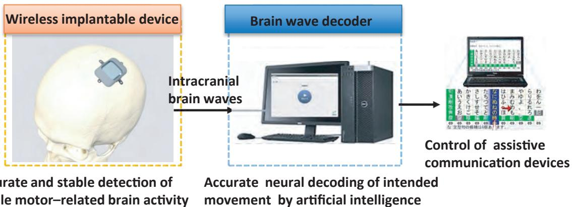
A brain-machine interface (BMI) is a technology used to read the contents of motions and communication from brain signals and to control robot arms and communication devices. This is expected as a technology to restore the impaired functions of disable people. In this project, we aim to perform a clinical trial of an implantable BMI device that records accurate brain waves using brain surface electrodes and to license it to a medical company.
