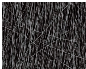
SEM image of poly( \epsilon -caprolactone) (PCL)-based electrospun scaffold
